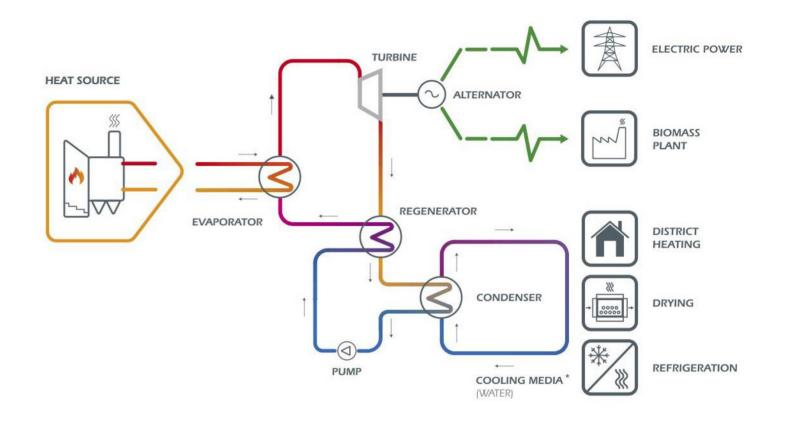
\*In **Heat Energy Generator**-only units, in which thermal users are not present, the cooling media can be either water or air with air cooled condensers.
