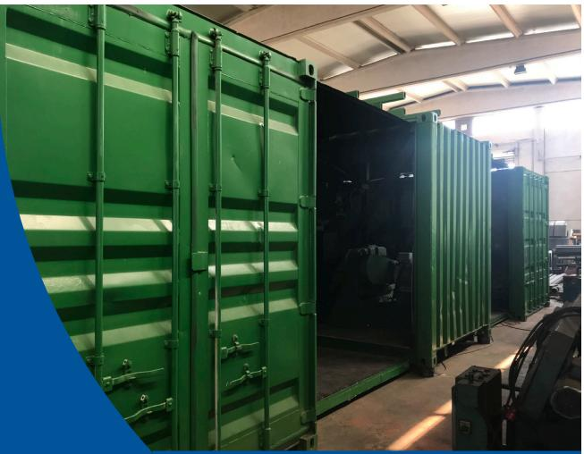
All 3 ton triple deck Total Waste Systems are housed in four parallel transport ready containers 40' x 8' (12.2M x 2.4M).
