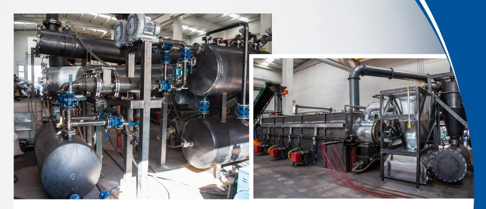
The "PyroOil" gets generated from the processed Geodyn pellets inside the reactors and transfers from the valves through the container. The containers next to the "PyroOil" generator are tanks that produce biochar or carbon black. The propane gas system is initialized for the first 60 minutes through six opposing burners till the temperature rises to 600 degrees Celsius. Then production of the 'Geodyn Generated SynGas' will engage the engine to run the generator.
