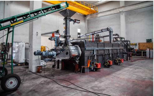
The Geodyn pellets are transferred to double reactors through the double air locks by cutting off the oxygen supply.
