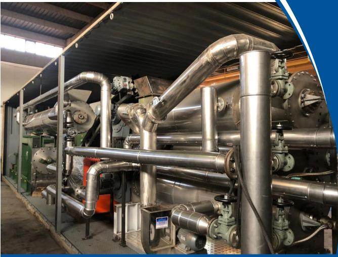
*This container houses the radiant heat processor which eliminates pathogens and eliminates odor. Next, the press will remove the liquid and transfer fluids to the filtration system.*
