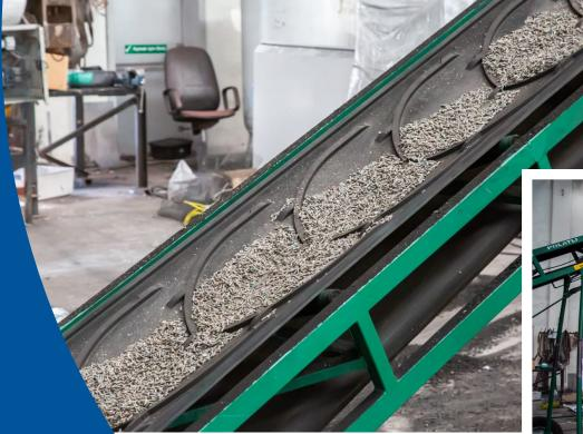
*Transferring the Geodyn pellets from the tripledeck on a conveyor to the pyrolysis system.*
